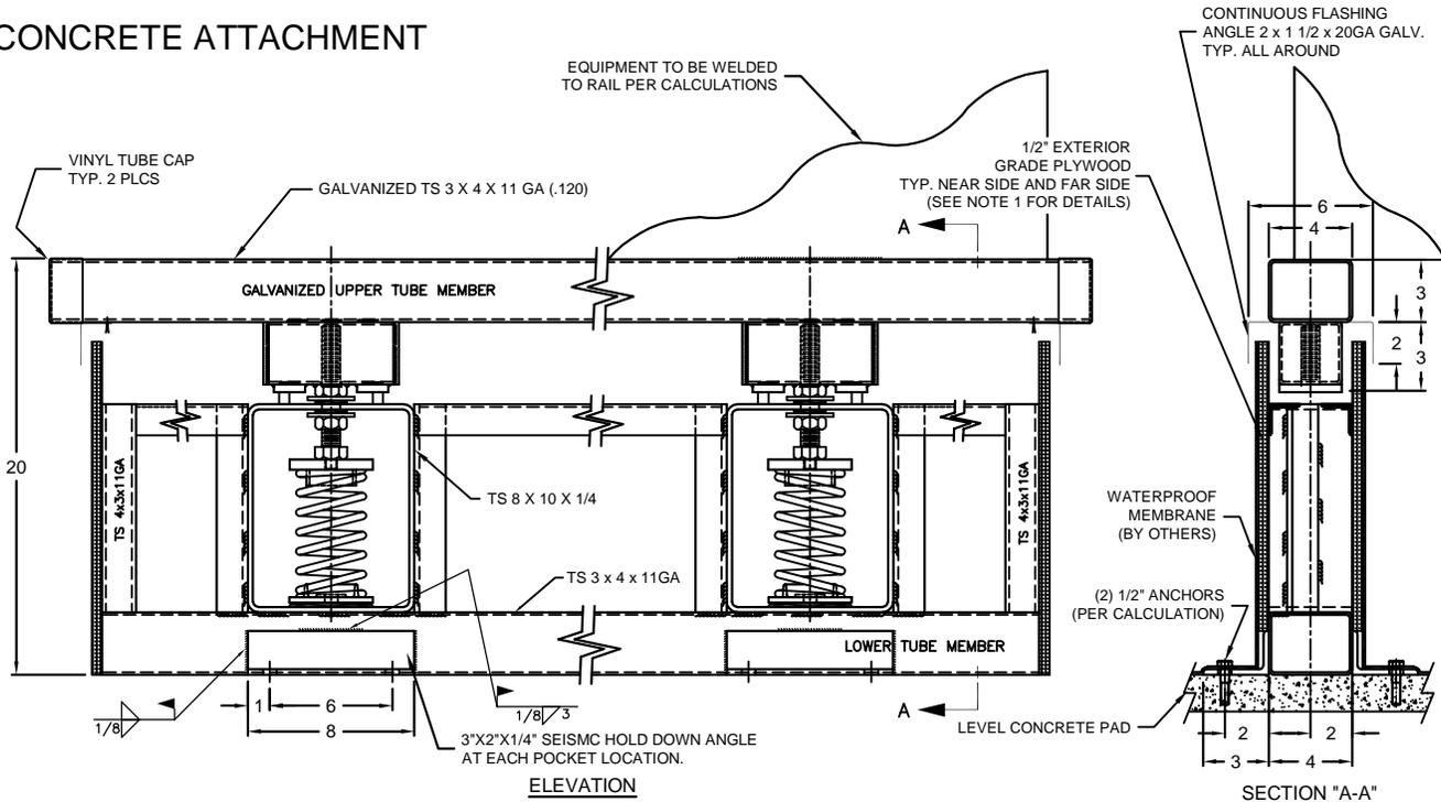
NOTE 1: ONE (1) PLYWOOD FASCIA TO HAVE CUT-OUTS MATCHING SPRING POCKET LOCATIONS. THE REMAINING FASCIA TO BE WITHOUT CUTOUTS.
