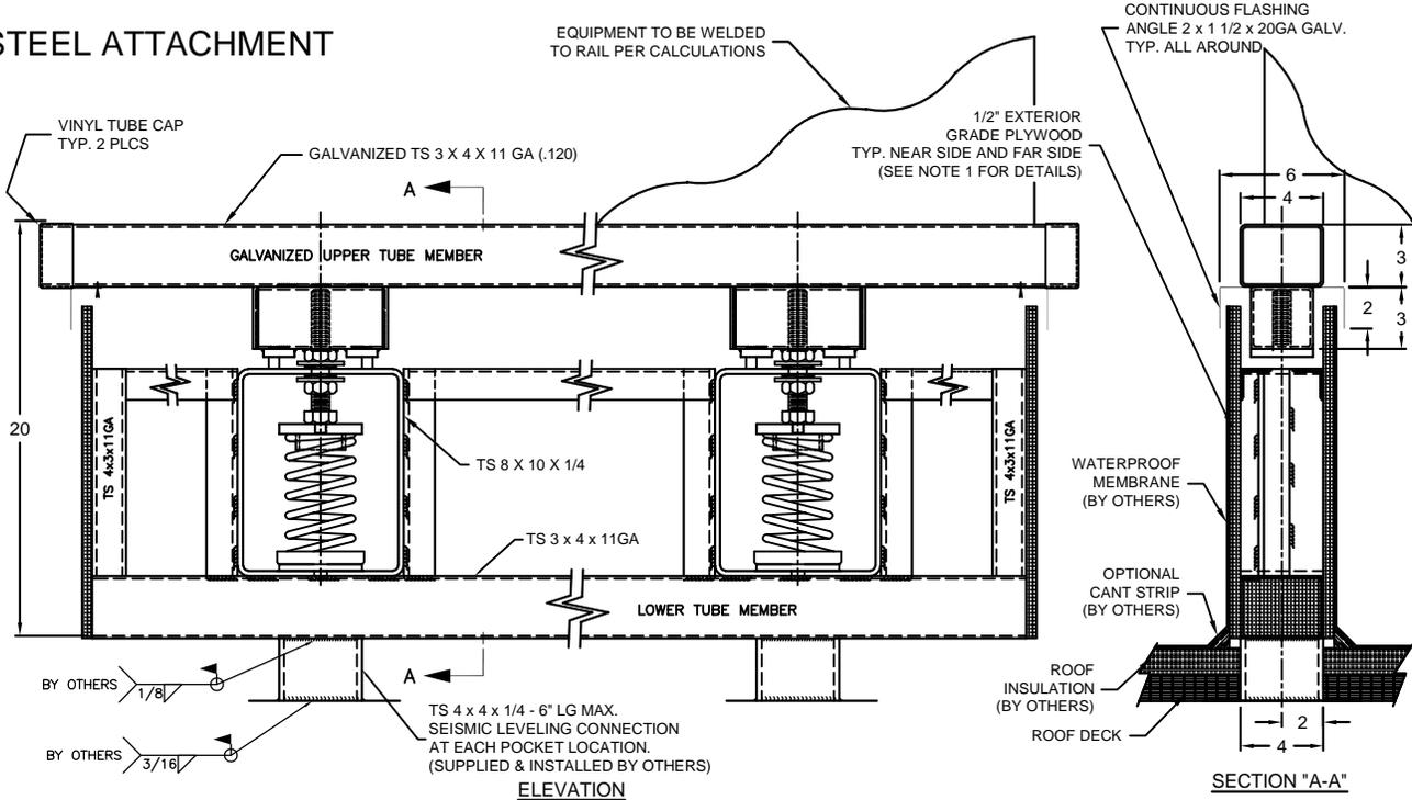
NOTE 1: ONE (1) PLYWOOD FASCIA TO HAVE CUT-OUTS MATCHING SPRING POCKET LOCATIONS. THE REMAINING FASCIA TO BE WITHOUT CUTOUTS.
